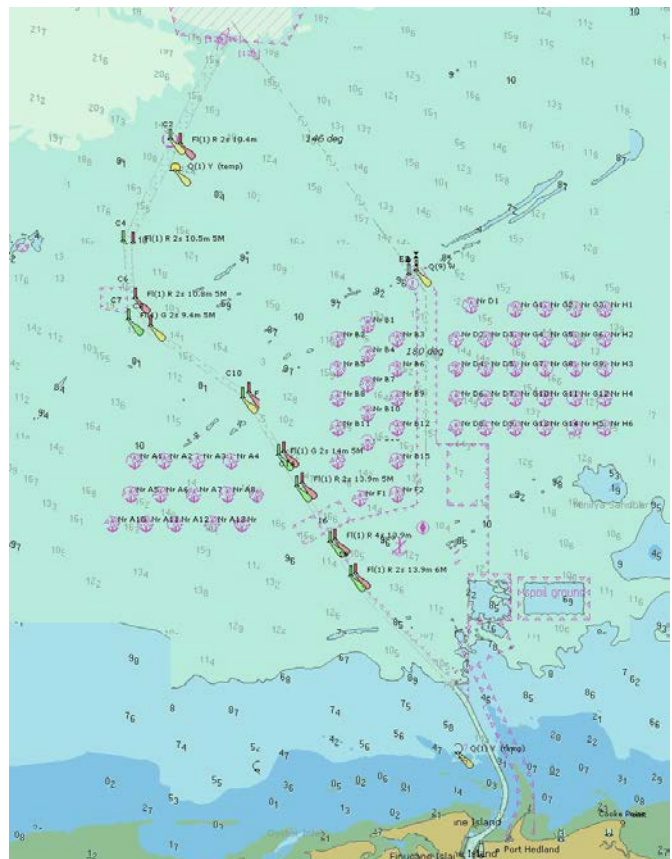
Figure 6 Channel Layout. The 42km, uni-directional, tidally restricted channel creates a challenging operating environment.
