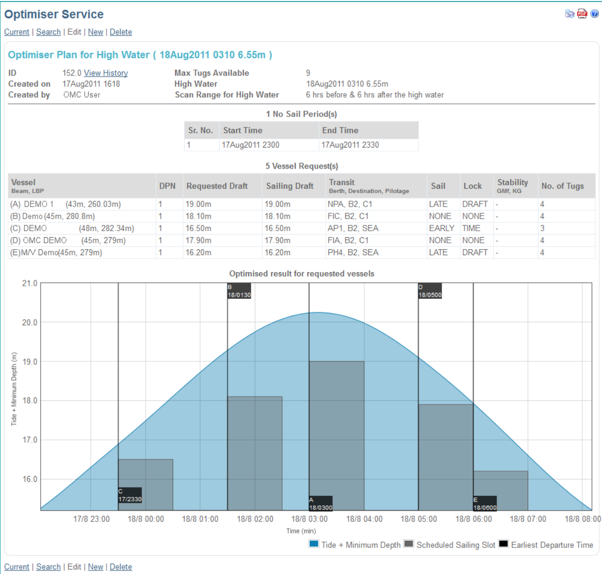
Figure 5 Sample output screen for the departure of multiple vessels on a tide.
