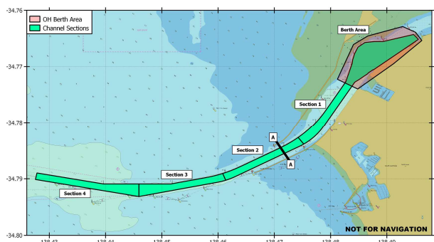
Figure 4 Independent sections analysed for vessel proximity to bounds. Channel cross section from Section 3.2.2 marked A-A [3]
